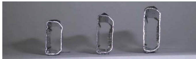
Figure 9: D-shape steel spacers of heights 13.5 mm, 17.5 mm, 15.5 mm
