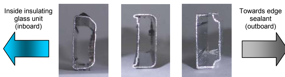
Figure 3 : Edge seal spacer designs: Left side visible inside insulating glass unit.
