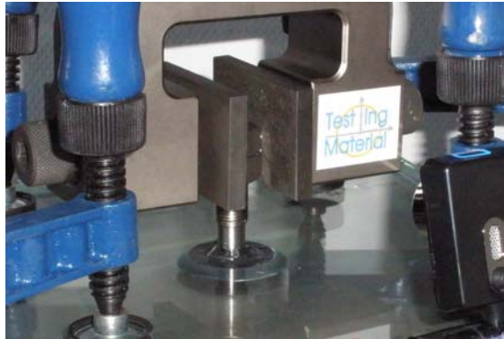
Figure 11: Test set-up for point support P1.
