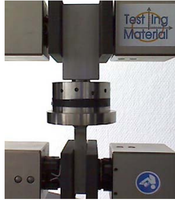
Figure 2: Photograph of point support specimen.
